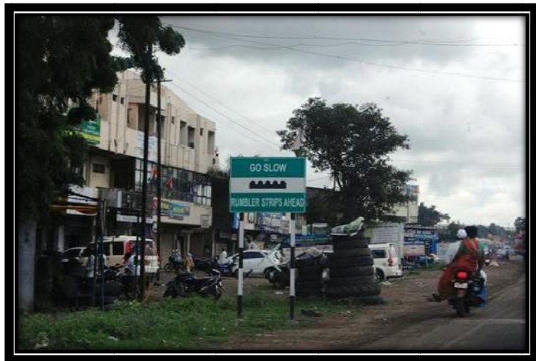
A speed breaker sign on a National Highway, with a non-conforming green background.
