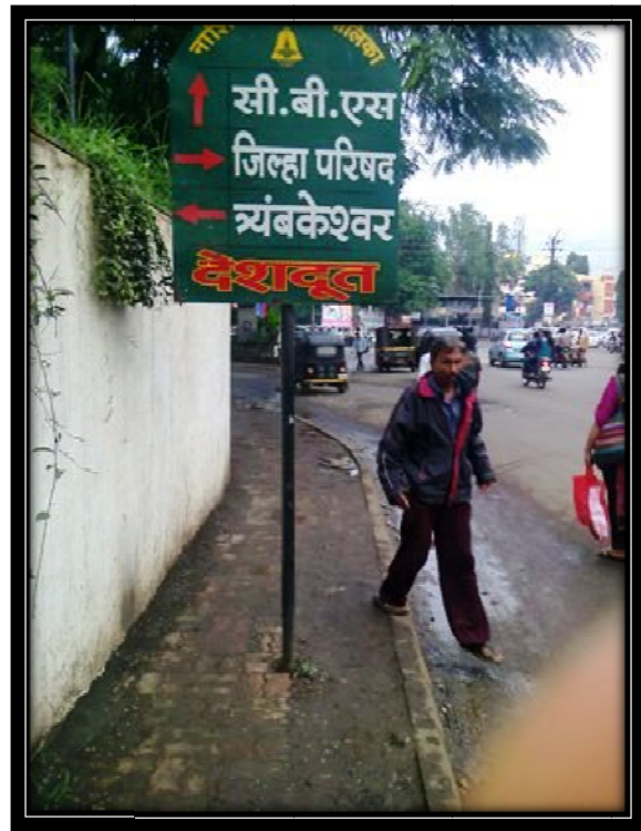
A sign in Nashik with a very small clearance from ground, forcing the pedestrian to get down from the footpath.
